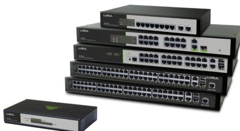
The Luxul XMS Gigabit Managed Switches feature front panel ports and front facing LEDs for simple connection and cable management. It's an excellent choice for expanding your network when using PoE-enabled devices such as VoIP, IP cameras and wireless access points.
