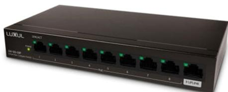
The SW-100 PoE+ unmanaged switches are small form factor network switches, with PoE+ ports capable of Gb Ethernet connectivity.
